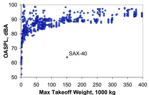
**Figure 3: Over All Sound Pressure Level at 2 km from touchdown for all Stage-3 certified aircraft<sup>18</sup> compared to estimate for SAX40 on a 3.0° approach.**
