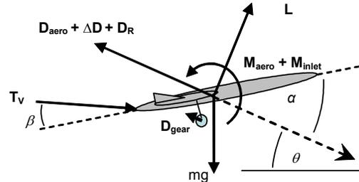
Figure 7: Aircraft force balance during a steady approach.
