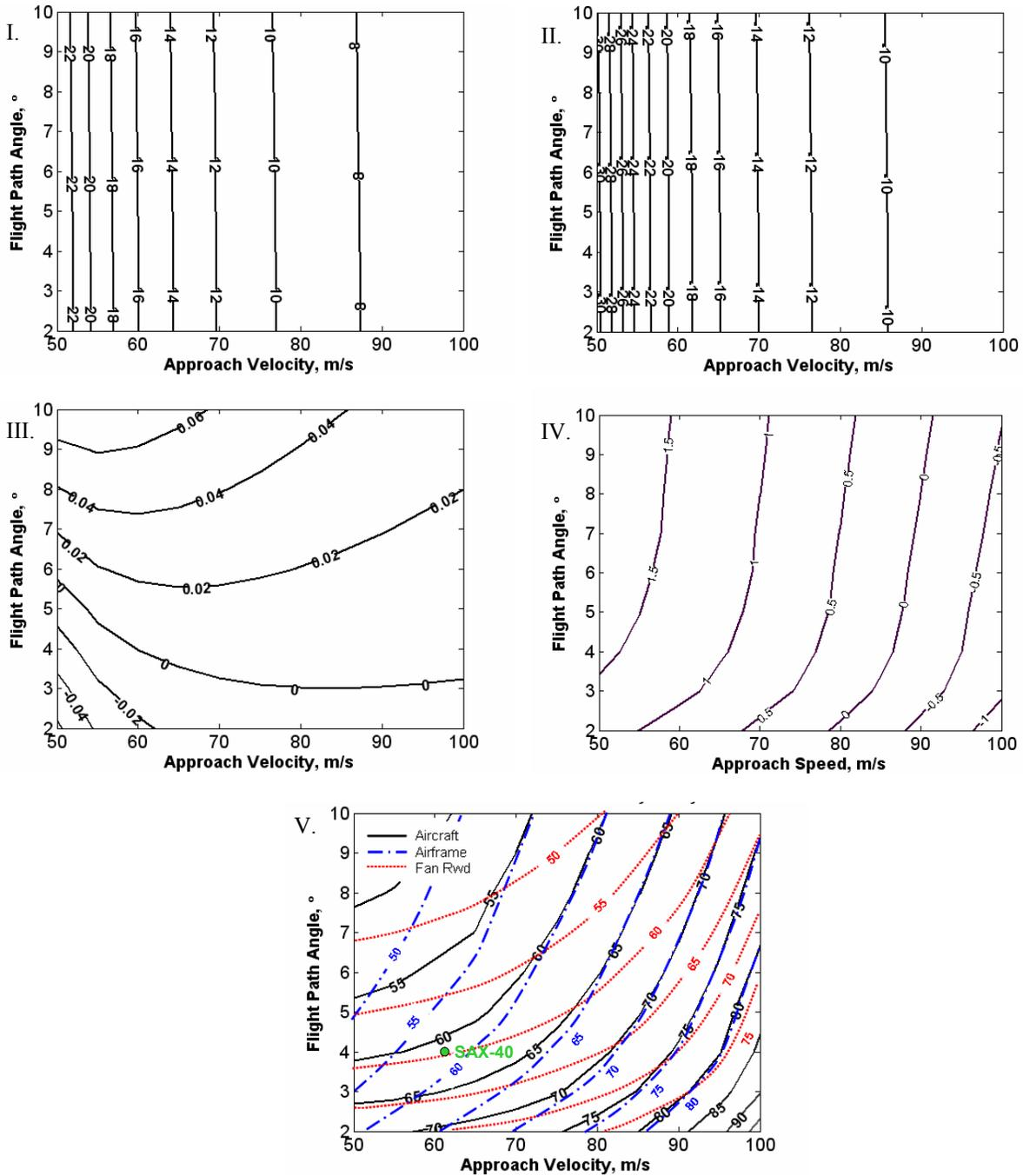
Figure 8: Impact of approach trajectory on SAX-40 (I) angle of attack, (II) elevator deflection, (III) change in drag to trim the aircraft, (IV) feasible landing threshold displacement (in km) on the 3 km design runway, and (V) aircraft noise at the airport perimeter with components from airframe and fan rearward.
