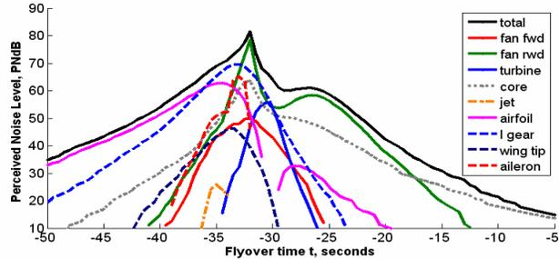
Figure 6: SAX-40 perceived noise level used in calculation of EPNdB. Time is relative to aircraft touching down 2 km from observer.
