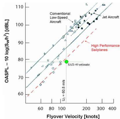
**Figure 5: Airfoil self-noise normalized by wing area and height as a function of velocity. Data from Fink.<sup>24</sup>**
