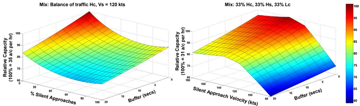
**Figure 13: Capacity analysis of ATC-imposed buffer, proportion & velocity of silent approaches.**
