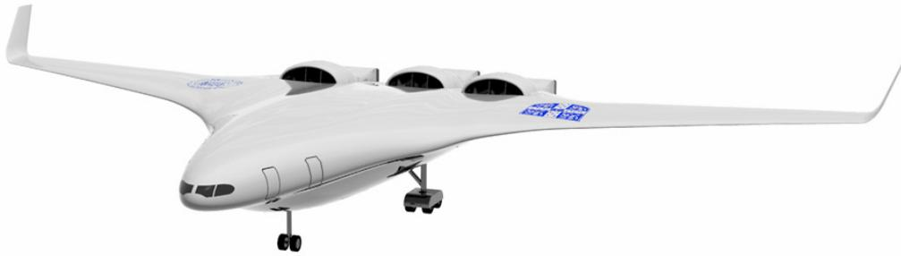
**Figure 1: Silent Aircraft eXperimental design SAX-40.**
