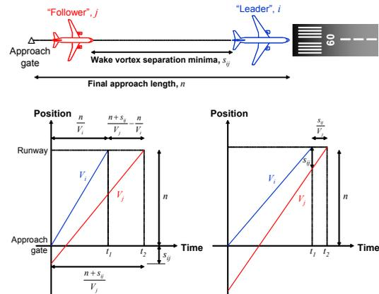
**Figure 12: Graphical representation of opening (left) and closing (right) approach cases. Adapted from <sup>44</sup>.**
