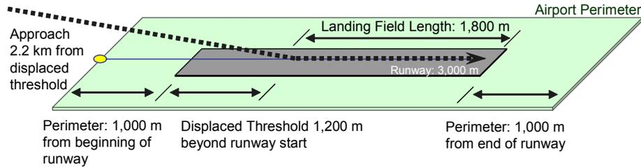
**Figure 4: Hypothetical airport dimensions used for the SAX-40 approach noise estimate.**
