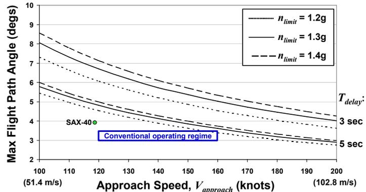
Figure 11: Results from SAX-40 go-around analysis with range of current operations.
