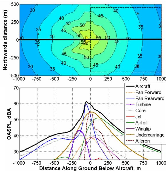
**Figure 3: Estimated SAX-40 approach noise footprint [top] and components [bottom] at airport perimeter.**
